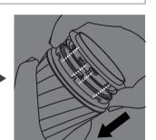
**Install Compression Unit** by inserting directly, all the way inside the Casing.
