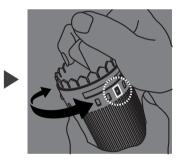
If not, hold Compressor Cover as shown and twist the Twist Compressor to bring the tab to the right-most hole.
