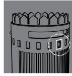
Remove Compression Unit and ensure the tab is in the right-most hole.
