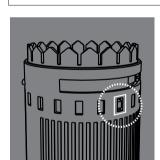
**Remove Compression** Unit and ensure the tab is in the right-most hole.
